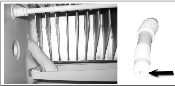
Check orifice diameter. Should be 1/4"
